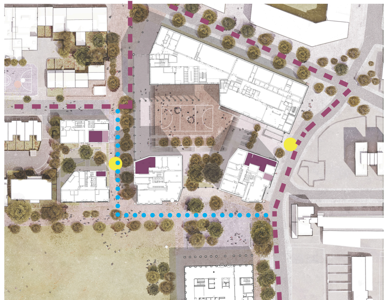
Ground Floor Level: Servicing and Waste Strategy
